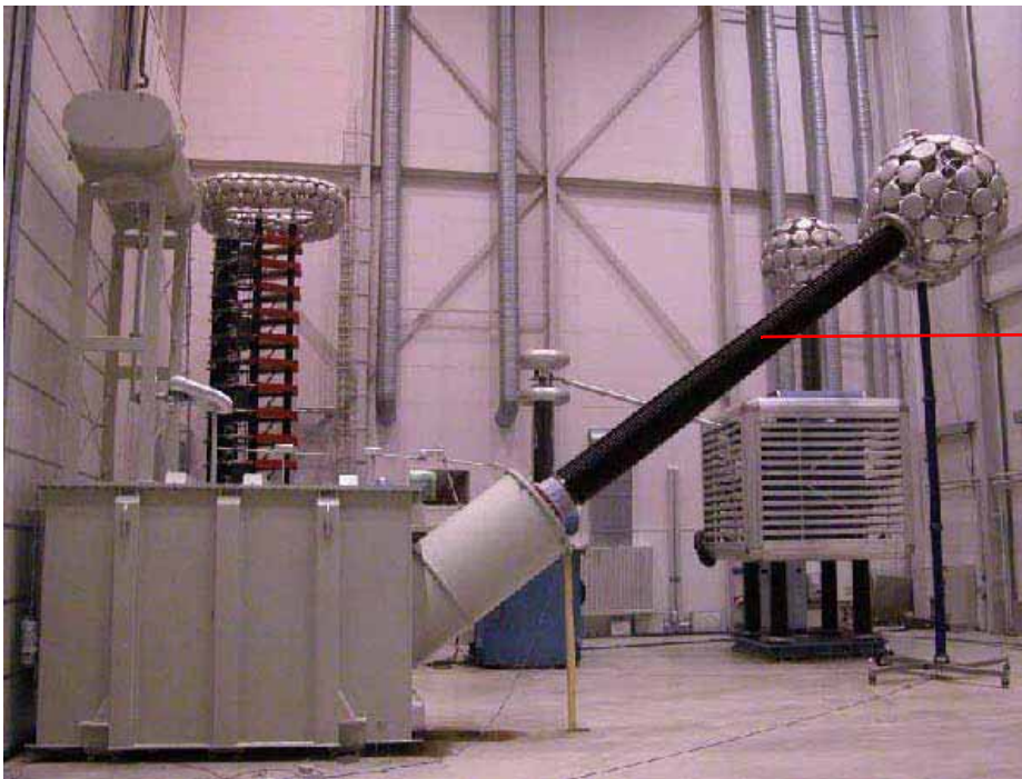
Transformer Bushing for 800 kV
